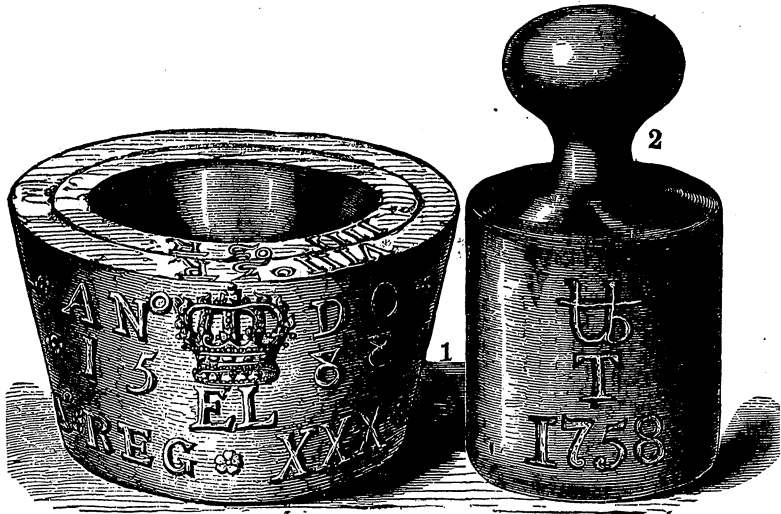
STANDARD ONE POUND TROY TEST WEIGHT.
